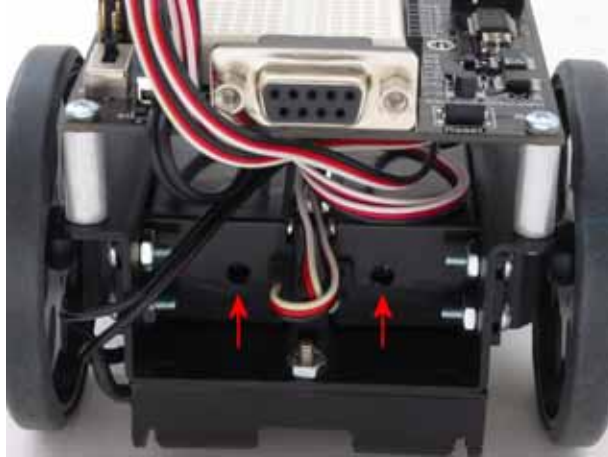
Figure 2.5: SumoBot Servo Adjustment Ports
